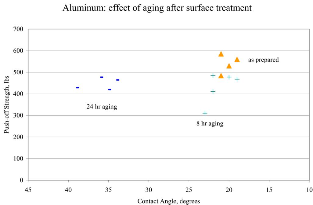
**Figure 6.** Push off load vs. contact angle for abraded and aged aluminum substrates.
